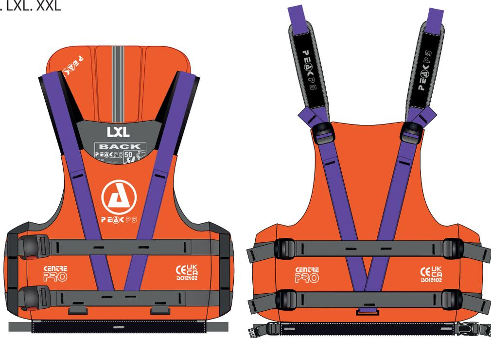
This PFD conforms to the standards EN ISO 12402-5:2020 and EN ISO 12402-6:2020 for personal flotation devices. PFD Type 50.
